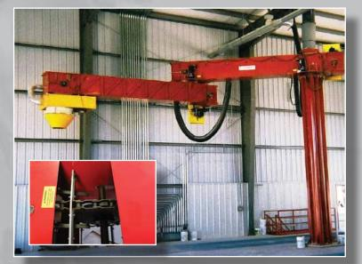
Like all DYNATEK loading systems, drag conveyor-based models are designed for articulated motion. Two slewing bearing-based pivots enable both conveyor arms to pivot separately resulting in nearly 330 degrees of rotation and loader reach of up to 27 feet. Loading is fast and convenient because you position the loader, not the truck, railcar or barge being loaded.
