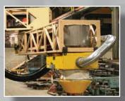
Retractable loading spouts with or without dust collection, insure precise, clean loading.
