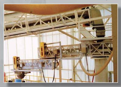
Like all DYNATEK loading systems, belt conveyor-based models are designed for articulated motion. Two slewing bearing-based pivots, enable both conveyor arms to pivot separately resulting in nearly 330 degrees of rotation and loader reach of up to 27 feet. Loading is fast and convenient because you position the loader, not the truck, railcar or barge being loaded.
