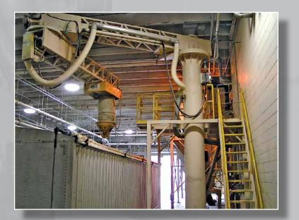
DYNATEK EconoLoader<sup>™</sup> Screw Conveyor loading systems are designed for maximum reliability. Materials of construction, slewing bearing ratings, pinion gears and drives are all carefully selected and the overall design is kept as simple as possible. The result – a service life of 25 years or more.
