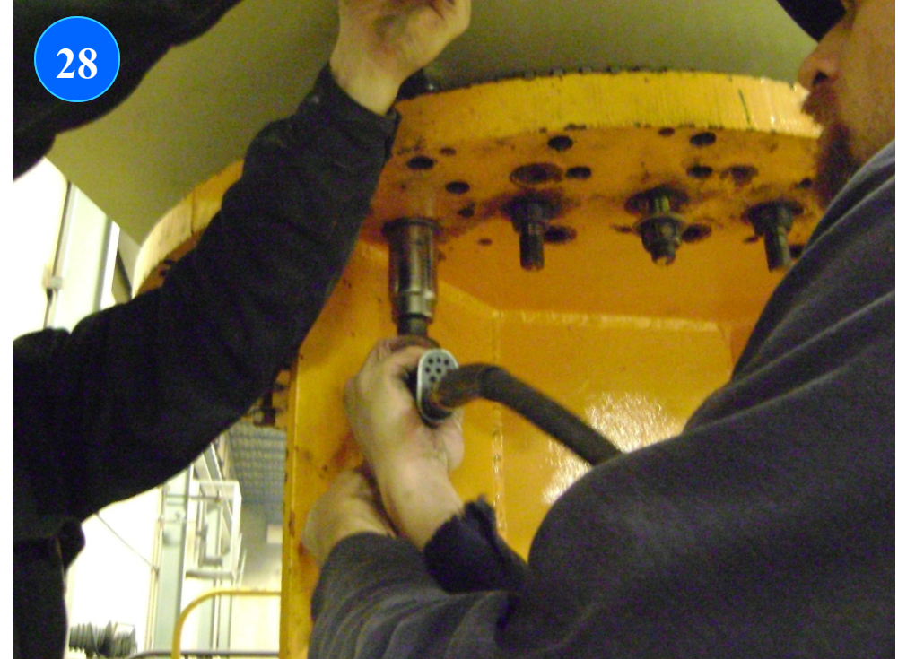
Use a 1 5/16" or 35mm open end flat wrench to tighten all the nuts.
