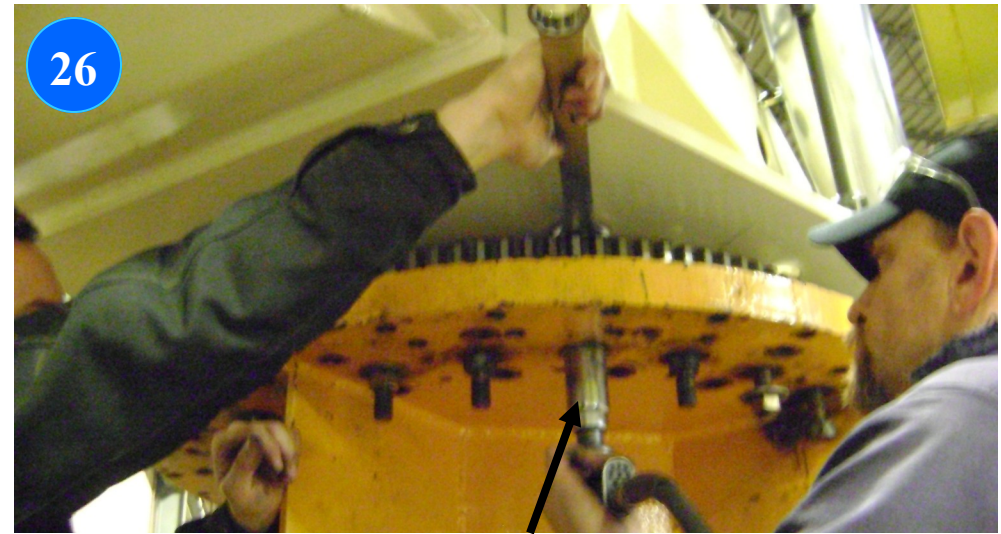
Use a 1 5/16" or 35mm deep well socket to tighten all the nuts.
