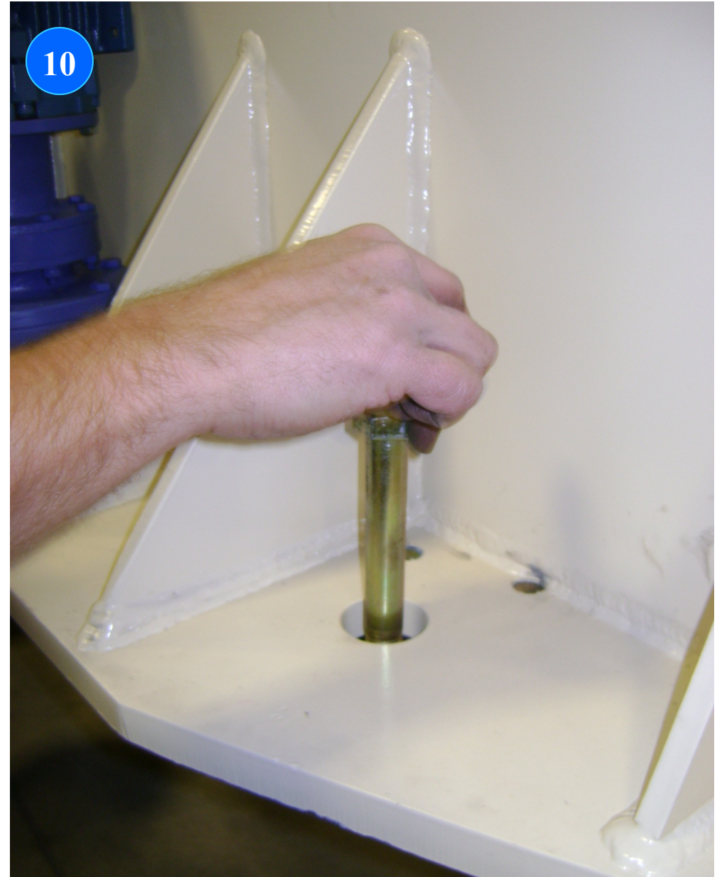
Drop 7/8-9x7" bolt into bearing
